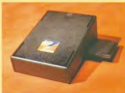
The Smart Stor is not a memory expansion, but a very small IDE interface with a hard drive mechanism.
